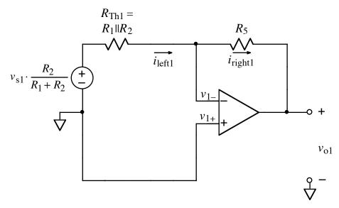
For this circuit,  $v_{1-} = v_{1+} = 0$  V. (The "1" stands for "case I".) Using  $v_{1-}$  to calculate  $i_{\text{left}1}$  and  $i_{\text{right}1}$  gives the following equation:
