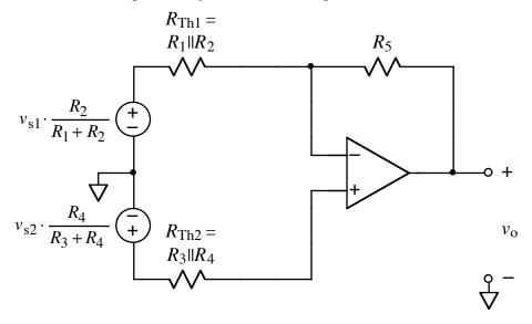
Since no current flows into the + input of the op-amp,  $R_{Th2}$  has no voltage drop and may be removed.
