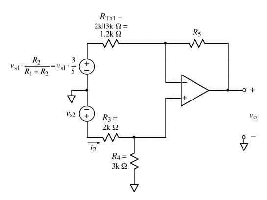
Likewise, converting the circuitry comprising  $v_{s2}$ ,  $R_3$ , and  $R_4$  into a Thevenin equivalent yields further simplification:
