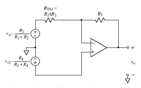
Now, applying superposition reveals that this circuit is a combination of a standard negative-gain circuit and positive-gain circuit.
