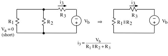
Our formula gives  $i_3 = \frac{V_b(R_1 + R_2)}{R_1R_2 + R_3(R_1 + R_2)}$  or  $i_3 = \frac{V_b}{R_1 ||R_2 + R_3}$ .
