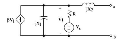
Construct a frequency-domain Thevenin's equivalent circuit at terminals **a** and **b**.
