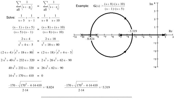
Breakaway (and arrival) points from the real axis ( $\sigma_b$ ) are also the solutions to:  $\frac{d}{ds}G(s) = 0$  where s is a real number (on the real axis) Why? Because gain =  $k = -\frac{1}{G(s)}$  The breakaway point will be the point between -5 and +1 with the highest gain. That is also the point with the lowest G(s) and highest - G(s). Either way  $\frac{d}{G(s)} = G(s)$
