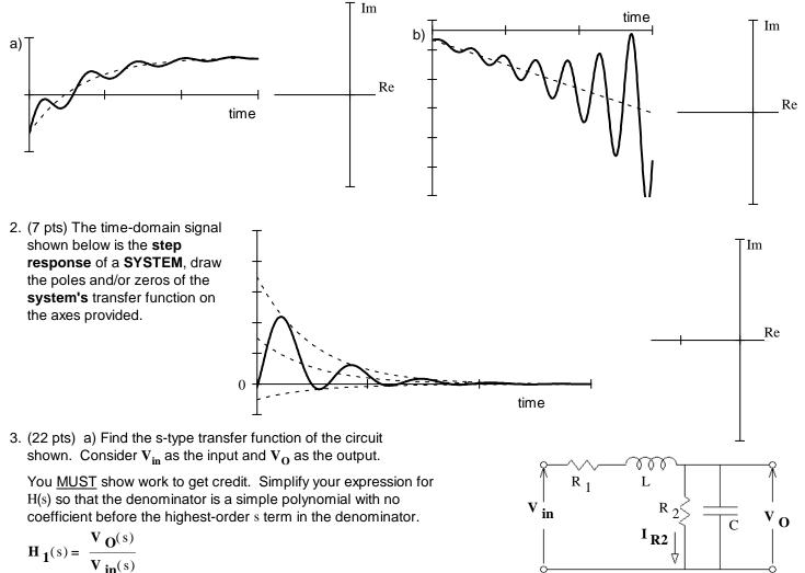
b) Modify the transfer function found in part a). Now consider  $I_{R2}$  as the "output".  $H_2(s) = \frac{I_{R2}(s)}{V_{in}(s)}$
