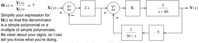
b) Find the value of K to make the transfer function (or part of it) critically damped.
