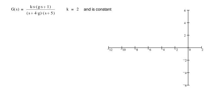
b) Draw an arrow to the place(s) on your root locus where you would like to place the closed-loop poles for minimal ringing and the shortest settling time. Extra credit if you find the value of g needed.
