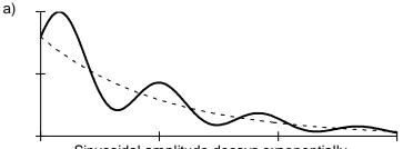
Sinusoidal amplitude decays exponentially
