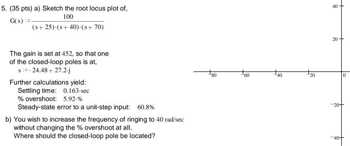
c) Add a LEAD compensator so that you will be able to place the closed-loop pole at the location found in b). Add the new zero at -30. Find the location of the new pole.
