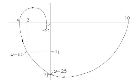
(6 pts) For the given Nyquist plot, find the gain margin and phase margin of the closed-loop system.
