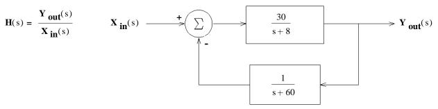
2. a) For the feedback system shown below, find the transfer function of the whole system, with feedback.
