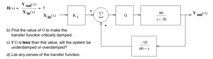
4. For the feedback system shown below, find the transfer function of the whole system, with feedback.
