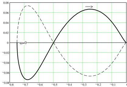
a) The Nyquist diagram for  $P(s)=5(s+2)/(s+1)^3$  is shown below (or in text), with the overall diagram shown on the left and the detail around the (-1,0) point shown on the right. Indicate what the gain margin and the phase margins are (for the phase margin, show work on the drawing below). Compare the gain margin results with those predicted by a root-locus plot or the Routh-Hurwitz criterion.
