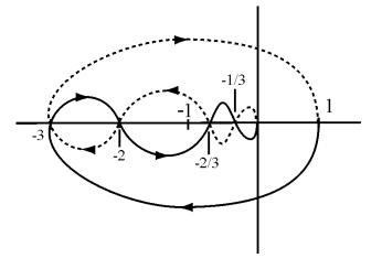
c) What are the values of the gain g > 0 by which the open-loop transfer function of part (b) may be multiplied, with the closed-loop system being stable?
