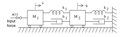
3. Find the equivalent electric circuit for the mechanical system shown. r(t) is an input. Show  $v_1$  &  $v_2$  on the circuit.
