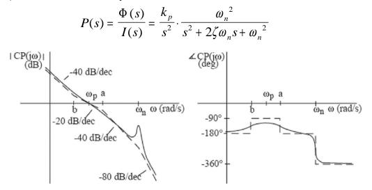
These are Bode plots of the loop transfer function for the approximate plant with the lead compensator. The magnitude plot shows as the crossover frequency, a condition that will be enforced by proper choice of the parameters. Assuming that  $\omega_n >> \omega_p$ , show that
