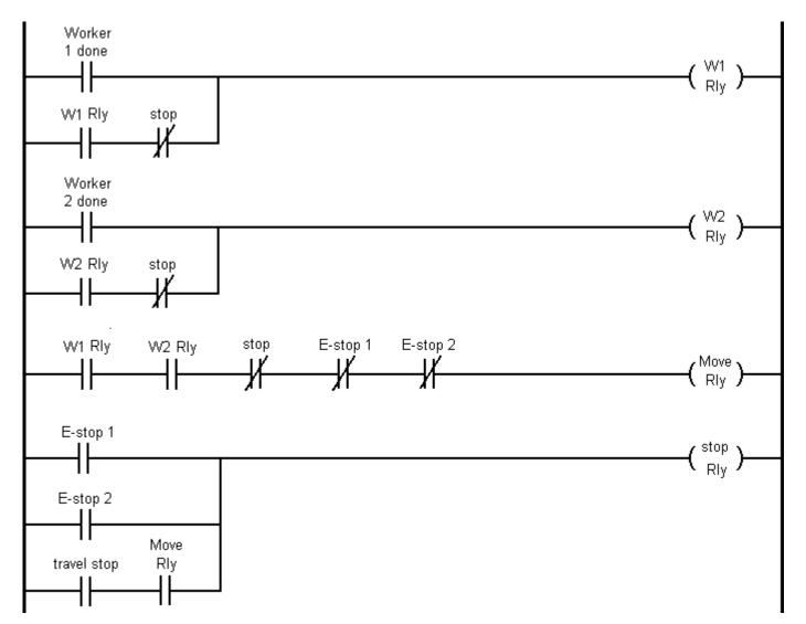
I've also added a "travel stop" input to stop the movement when the item reaches the next station and a reset method (which may not allow the next movement the unless you roll past the "travel stop" sensor). Also note that emergency stop buttons work in two ways, one of which does not rely on the stop relay.
