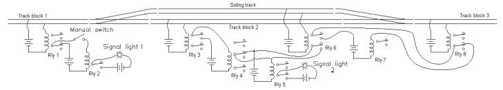
Relays can be hooked to one another and to other switches to create logic systems which which could operate signal lights or switch points or do many other things. But the logic is VERY hard to follow.
