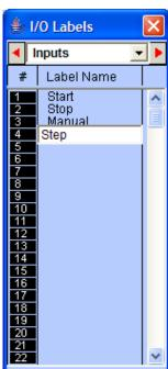
10. After entering label names for Inputs #1 to #4, move to the "Output" table by pressing the right cursor key or by clicking on the right arrow button. Enter all the output and relay label names in their respective I/O tables. We will discuss the "Timer" table in the next step.
